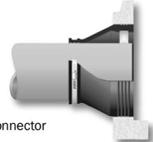
The 106 Series connector is 8 inches long, the 406 Series connector is 6 inches long. The number following the hyphen in our model numbers is the required hole size. The S106-20 Series is available in Stainless Steel Wedge only.
