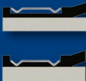
*Patented Waveband technology creates a more effective seal by concentrating the compressive force of the expansion band. The rubber is “captured” between the band and the concrete.*
